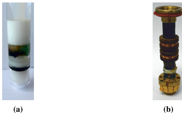
Figure 3.1: (a) Lymph node sample fixated with plastic system in glass tube. (b) VSM detection coil set with bore diameter 10.6 mm.
