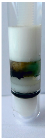
Figure 4.1: The sample holder used for VSM measurements of lymph nodes. The lymph node is placed in a glass tube between two Delrin parts. The length of the upper part is adjustable to allow for firm fixation of lymph nodes with different size.
